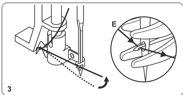
3. Take the thread in front of the needle and make sure it is under the hook pin (E). Then hold the thread slightly upwards so that it hangs on the hook.
