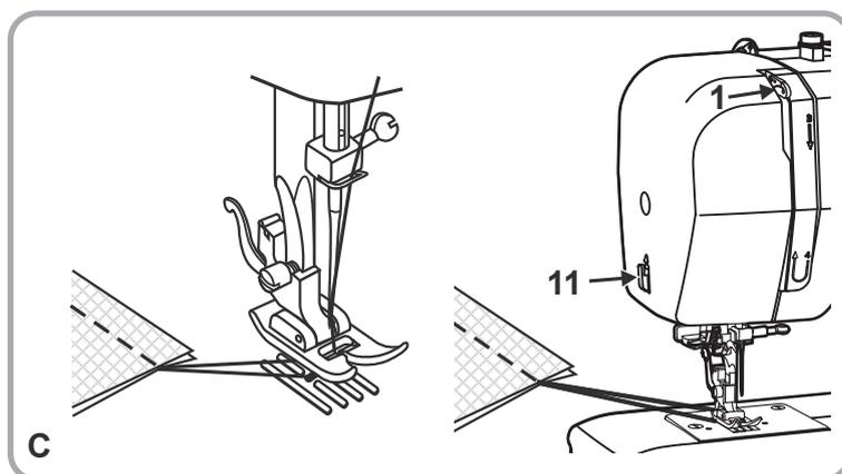
Reverse sewing is used to lock the threads in the beginning and at the end of the seam or wherever reinforcement is needed.
