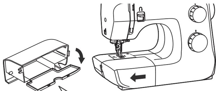
If you want to sew on the arm bed, pull out the snap-in sewing table (7) in the direction of the arrow.
