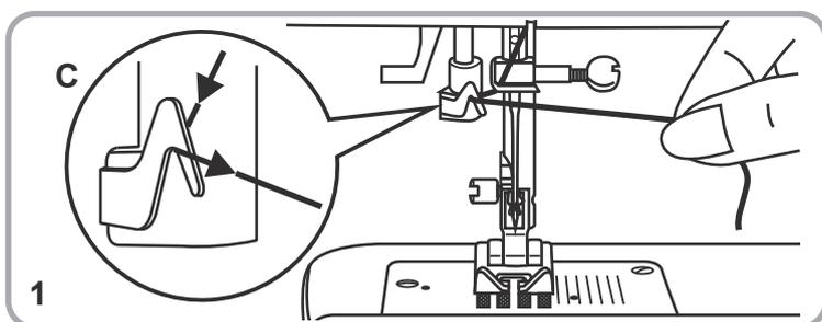
1. Lower the presser foot (9). Pass the thread around the thread guide (C).
