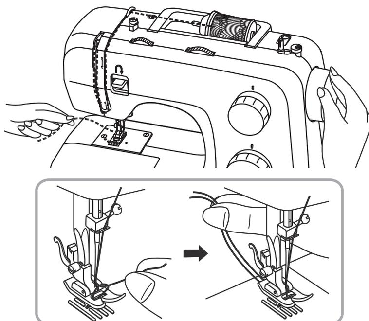
Hold the end of the upper thread with the left hand. Turn the handwheel (21) in the anticlockwise direction until the needle is again raised (a complete revolution).
