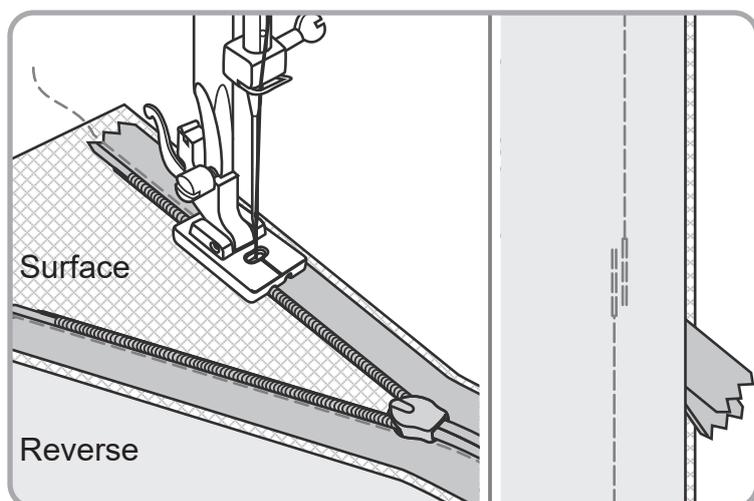
Close zipper. Slide zipper foot (c) to the left so that needle is in the outer notch. Pin the seam together below zipper opening. Fold end of zipper out of the way and lower the needle by hand slightly above and to the left of the last stitch.
